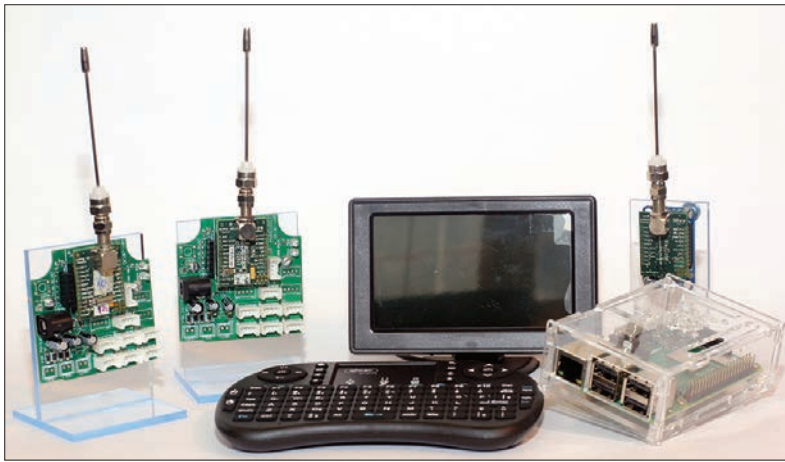
Figure 4. The open source IoT development kit used to illustrate the presentation of the implementation phase.
